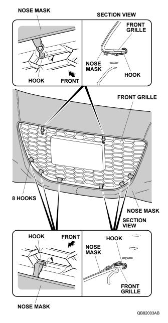
16. Close the hood, and adjust the position of the nose mask to the hood.
